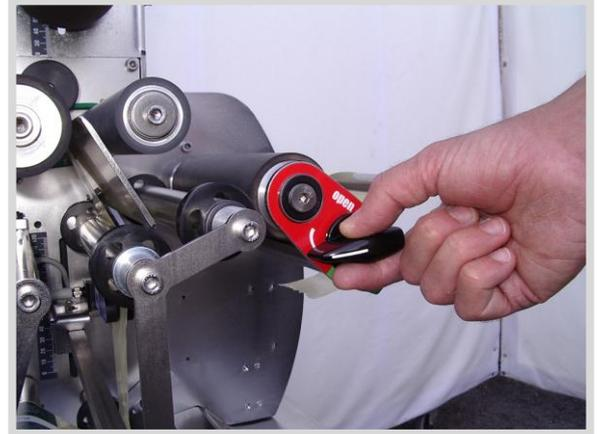
Photo 9.17 The knob being turned for blocking
