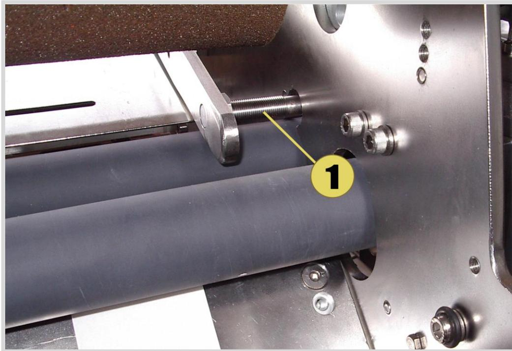
Photo 8.3 – Sensor for notch detection
