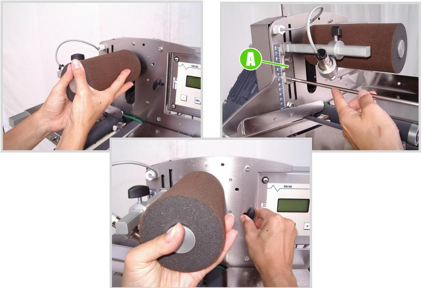
Photo 9.4 Container diameter adjustment
