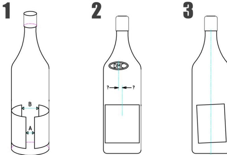
Figure 9.1 Corrections on cylindrical containers - Caption: 1) centering between label and back label 2) centering between label and spot 3) label alignment
