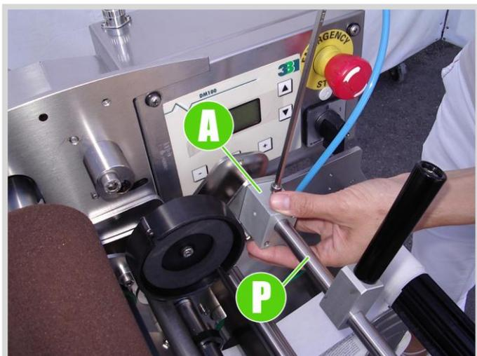
Photo 8.8 Adjusting label height from bottom
