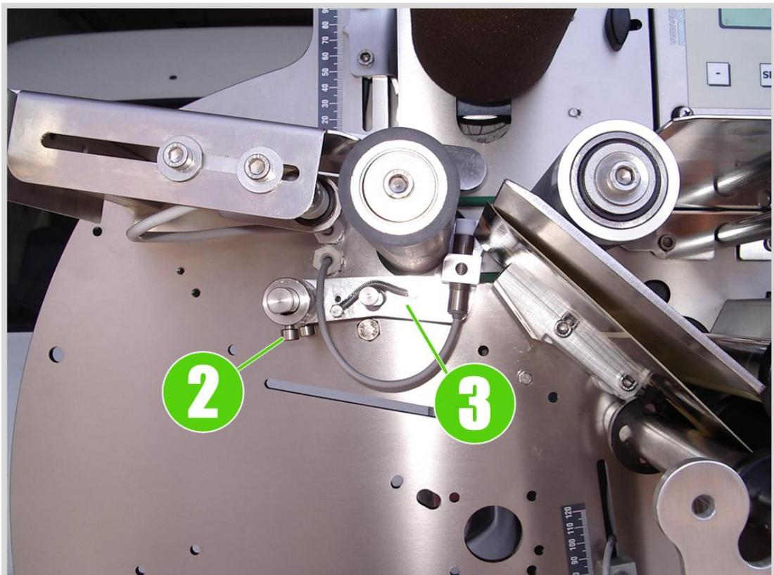
Photo 8.2 Support of the side-notch detection sensor
