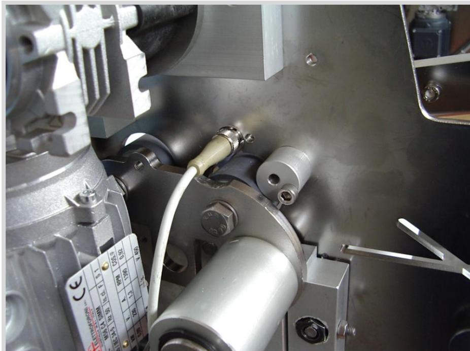
Photo 8.5 – Back view with notch detection connector
