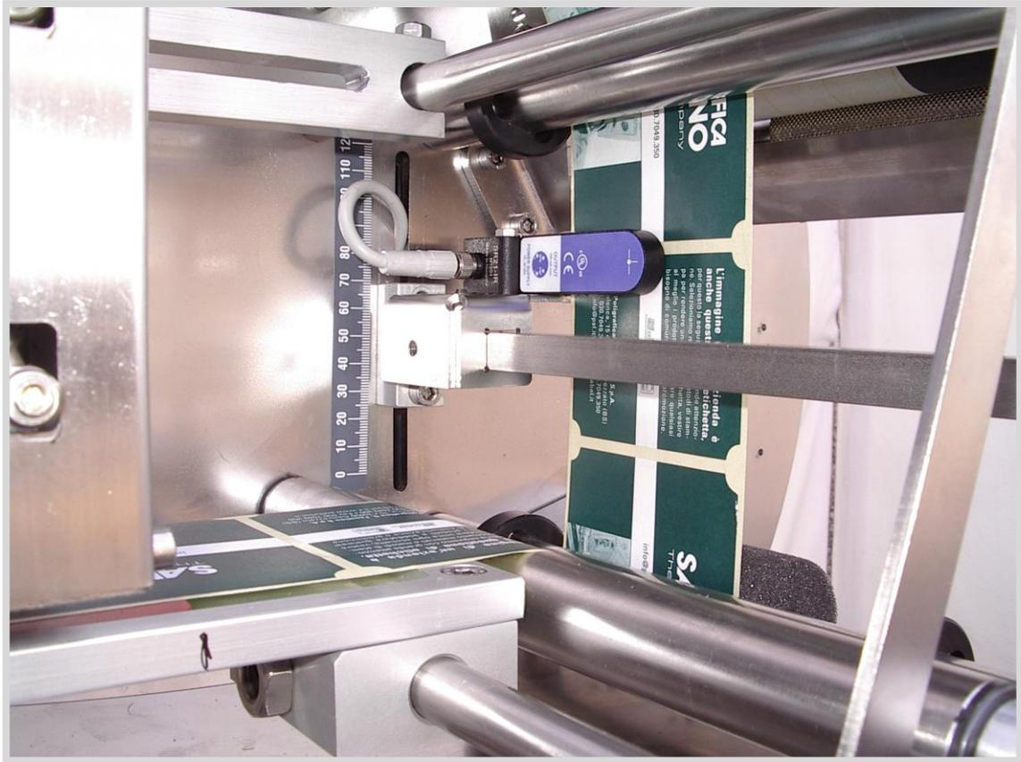
Photo 9.7 Reading position of the photocell
