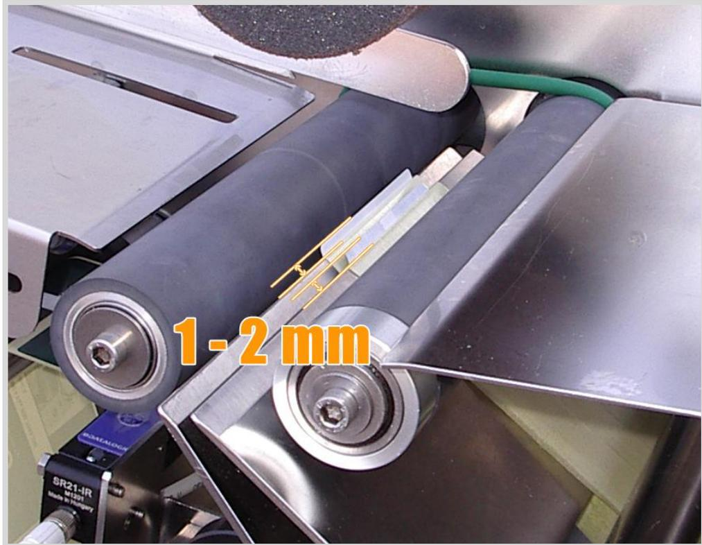
Photo 9.14 Correct label output from blade
