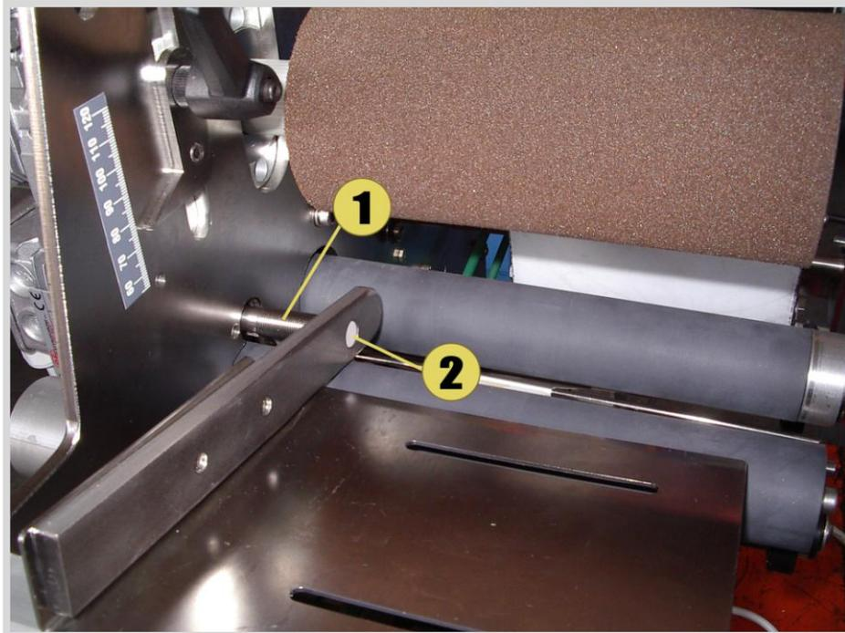
Photo 8.4 – key: 1) sensor 2) detection head
