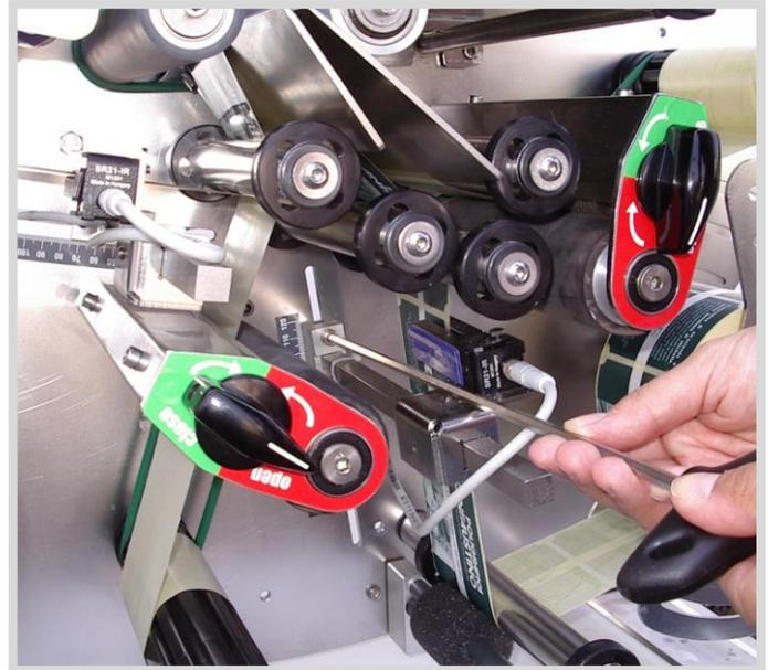
Photo 9.6B Right photocell adjustment
