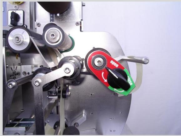
Photo 9.16 Rubber driving roller released (OPEN)
