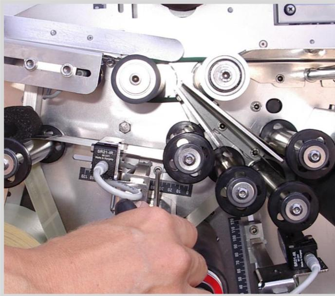
Photo 9.6A Left photocell adjustment
