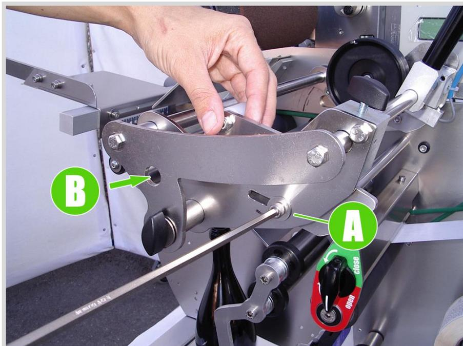
Photo 9.21 Adjustment of label alignment for square bottles
