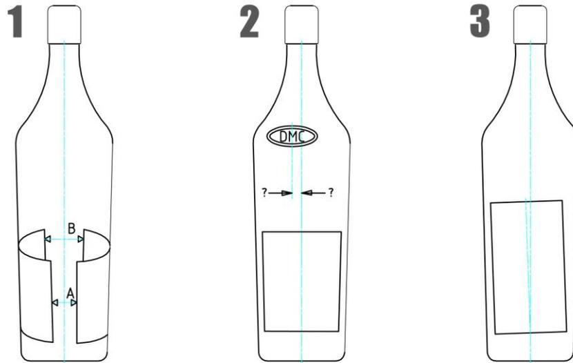
Figure 9.2 Adjustment on conical containers
