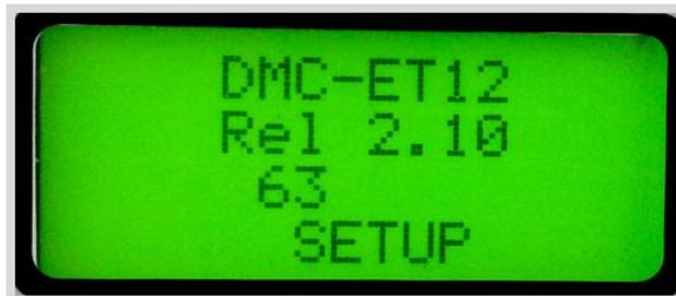
The value in the line above the word SETUP (pictured 63) is the global counter of bottles packed, non-editable by the customer: to reset this value you must access the data machine and set to line 1) LANGUAGE the special value 100, then leave the machine data, shut down the emergency button and restart.
