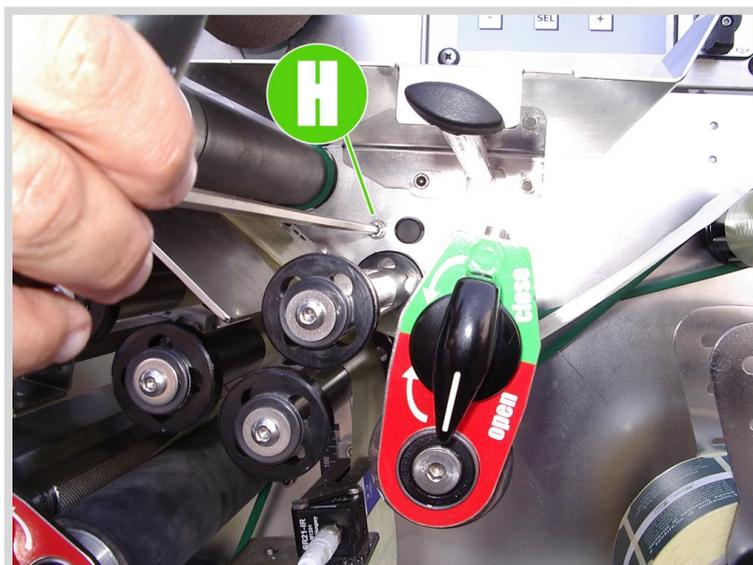
Photo 9.20 Label alignment on conical containers
