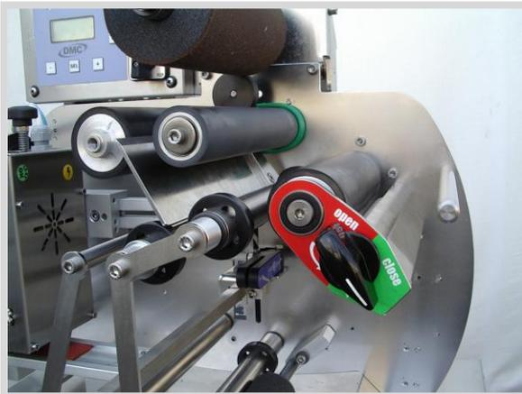
Photo 9.18 Rubber driving roller blocked (CLOSE)
