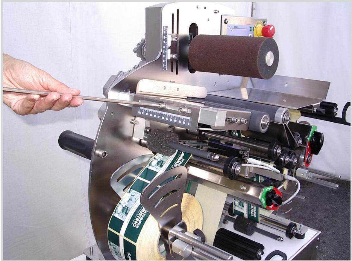
Photo 9.8 Adjusting label height from the bottom
