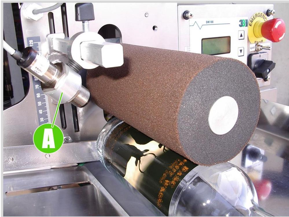
*Photo 8.1 Label detection photocell*
